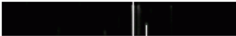
Fig. 5. Vertical edges symmetry: the horizontal axis represents the position of symmetry axis while the vertical axis represents the width of the symmetry box (small on the top and large on the bottom of the image).
